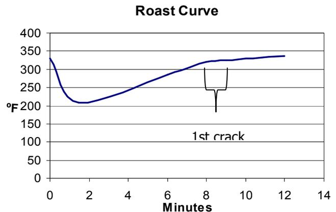
When the first crack begins the measuring device should read somewhere between 160°C – 163°C (320°F – 325°F). This first exothermic stage should last about two minutes. The ideal roast point is achieved after 11 to 12 minutes with a temperature of 168°C – 170°C (334°F – 338°F), and nearly 40 seconds after finishing the first crack. This roasting protocol should lead to a 55 Agtron (E20-CP) in whole bean and 60 Agtron in ground coffee.<sup>10</sup>
