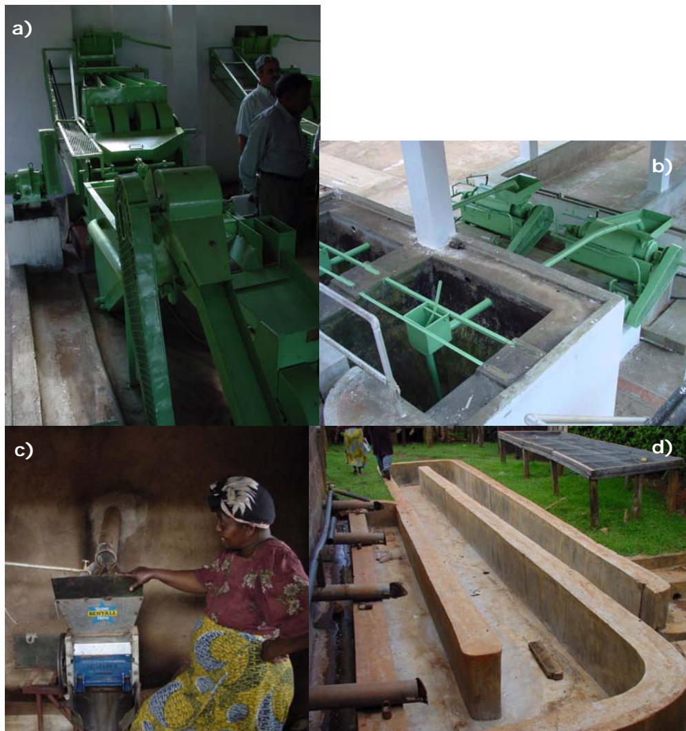
Fig. 2 - Some of the equipment and facilities required for wet processing: a) One of two disc pulpers, on a large estate, b) Siphon tanks, aqua-washers, soaking tanks, on a large estate, c) Smallholder pulper, d) Smallholder washing channels and table dryer
