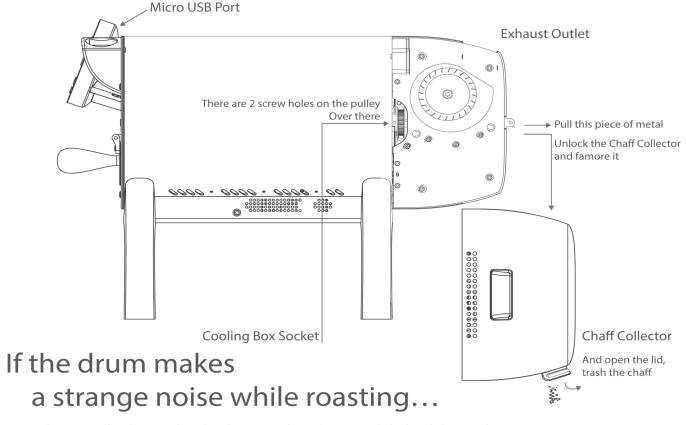
A grinding sound indicates that the drum may have become dislodged during shipping. Make sure the gap between the pulley and the housing is approximately 1 mm. You can adjust the gap by loosening the two screws on the pulley and pulling the drum into place before refastening.
